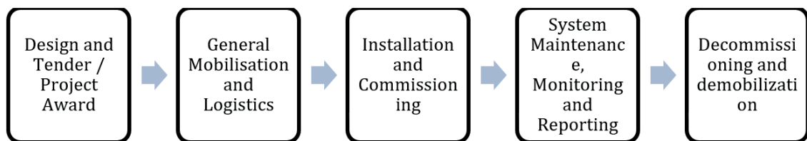
Figure 3. Typical flow process chart for a construction dewatering/groundwater control project.
